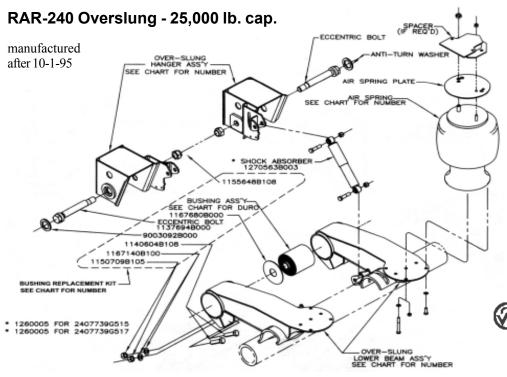
NOTICE: SUSPENSION IDENTIFICATION: Ridewell Suspensions are identified by a metal tag that indicates part number, capacity and serial number. Consult your trailer manufacturer for your correct mounting height.
