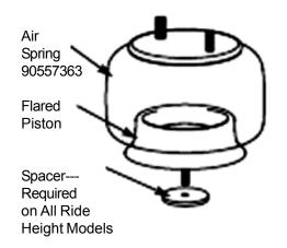
IMPORTANT: Air Springs and spacers must not be mixed on the same axle, and the proper spacers must be used on the new air springs.
