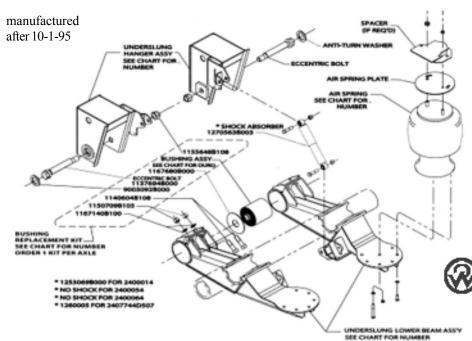
NOTICE: SUSPENSION IDENTIFICATION: Ridewell Suspensions are identified by a metal tag that indicates part number, capacity and serial number. Consult your trailer manufacturer for your correct mounting height.
